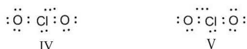
Figure 4: Structures of \text{ClO}_2 in terms of three-electron bond. Form IV and V are the structural twists of three electrons between the two oxygen atoms
