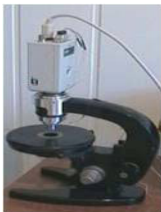
Figure 12: A model of an old capillary scanner (the 60's of the 20th century) with the first attempt to take video, which became a prototype for digital optical capillaroscopy.
